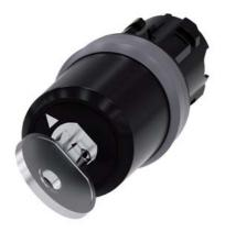
key-operated switch Siemens, 22 mm, round, plastic with metal front ring, lock no. LSG1, with 2 keys, 2 switch positions O<I, momentary contact type, actuating angle  $45^{\circ}$ , 10:30h/12h, key removal O, with laser labeling, lower case
