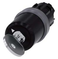
Key-operated switch BKS, 22 mm, round, plastic with metal front ring, lock number S1, with 2 keys, 2 switch positions O-I, latching, actuating angle  $90^{\circ}$ , 10:30h/13:30h, key removal O+I, with laser labeling, lower case
