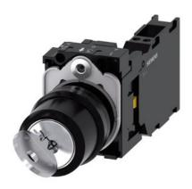
RONIS key-operated switch, 22 mm, round, plastic, lock number SB30, with 2 keys, 2 switch positions O-I, latching, 10:30h/13:30h, with holder, 2 x 1 NC with mounting monitoring, spring-type terminal, possible special locks: SB31, 421, 455
