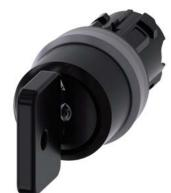
Key-operated switch O.M.R, 22 mm, round, plastic with metal front ring, lock number 73034, black, with 2 keys, 3 switch positions I-O-II, latching, actuating angle 2x45°, 10:30h/12h/13:30h, Key removal I+O+II, with laser labeling, upper case and lower case, always upper case at the beginning of the word
