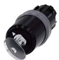
key-operated switch Siemens, 22 mm, round, plastic with metal front ring, lock number SSG10, with 2 keys, 2 switch positions O-I, latching, actuating angle 90°, 10:30h/13:30h, key removal O+I, Z=50-unit packaging
