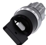
key-operated switch Siemens, 22 mm, round, metal, shiny, lock no. VL5, with 2 keys, 2 switch positions O<I, momentary contact type, actuating angle 45°, 10:30h/12h, key removal O, with laser labeling, upper case
