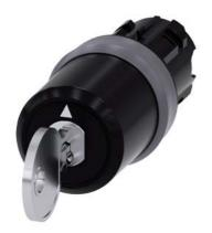
key-operated switch Siemens, 22 mm, round, plastic with metal front ring, lock number SSG10, with 2 keys, 3 switch positions I>O<II, momentary contact on the left, latching on the right, actuating angle  $2x45^\circ$ , 10:30h/12h/13:30h, key removal II, with laser labeling, lower case
