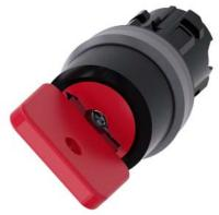
Key-operated switch O.M.R, 22 mm, round, plastic with metal front ring, lock number 73037, red, with 2 keys, 2 switch positions O<I, momentary contact type, Actuating angle 45°, 10:30h/12h, key removal O, with laser labeling, upper case
