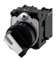
Selector switch, illuminable, 22 mm, round, plastic, white, selector switch, short, 2 switch positions O-I, latching, 10:30h/13:30h, with holder, 1 NO, 1 NC, screw terminal, with laser labeling, upper case and lower case, always upper case at beginning of line
