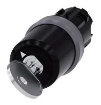
Key-operated switch BKS, 22 mm, round, plastic with metal front ring, lock number S1, with 2 keys, 2 switch positions O<I, momentary contact type, Actuating angle 45°, 10:30h/12h, key removal O, with laser labeling, upper case and lower case, always upper case at the beginning of the word
