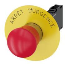
EMERGENCY STOP mushroom pushbutton, 22 mm, round, metal, shiny, red, 40 mm, positive latching, acc. to EN ISO 13850, rotate-to-unlatch, with yellow backing plate, inscription: Arrêt d'urgence, with holder, 1 NO+1 NC, screw terminal, Z=20-unit packaging
