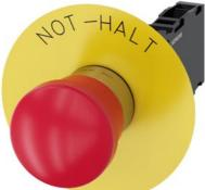
EMERGENCY STOP mushroom-type actuator, 22 mm, round, metal, shiny, red, 40 mm, positive latching, according to EN ISO 13850, pull-to-unlatch mechanism, with yellow backing plate, inscription: NOT-HALT, with holder, 1 NO+1 NC, screw terminal, Z=20-unit packaging
