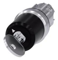
key-operated switch Siemens with key monitoring, 22 mm, round, metal shiny, lock number SSG10 with 2 keys, 2 switch positions O-I, latching, actuating angle 90°, 10:30h/13:30h, key removal/ejection in O, Z=50-unit packaging
