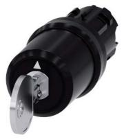
Key-operated switch BKS, 22 mm, round, plastic, lock number S1, with 2 keys, 3 switch positions >O<II, momentary contact type, actuating angle  $2x45^\circ$ , 10:30h/12h/13:30h, key removal O, with laser labeling, upper case and lower case, always upper case at beginning of line
