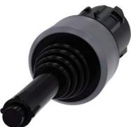
Coordinate switch, 22 mm, round, plastic with metal front ring, black, 2 switch positions, vertical latching, with mechanical interlocking, with laser labeling, inscription or symbol, Customer-specific selection with SIRIUS ACT configurator (CIN)
