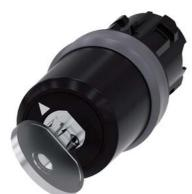
Key-operated switch BKS, 22 mm, round, plastic with metal front ring, lock number S1, with 2 keys, 2 switch positions O-I, latching, actuating angle 90°, 10:30h/13:30h, key removal O, with laser labeling, upper case and lower case, always upper case at the beginning of the word
