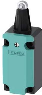
Position switch Metal enclosure 40 mm according to EN 50041 Roller plunger with Stainless steel roller 13 mm, 3 mm overtravel, 1 NO/1 NC quick action contacts, Device connection 1x (M20 x 1.5), actuating/restoring force 30 N only available as complete unit
