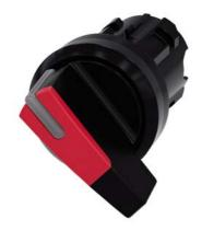
Selector switch, illuminable, 22 mm, round, plastic, red, selector switch, long, 2 switch positions O-I, latching, actuating angle 90°, 10:30h/13:30h, with laser labeling, upper case
