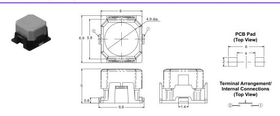
Note: Unless otherwise specified, a tolerance of ±0.4 mm applies to all dimensions. No terminal numbers are indicated on the Switches.
