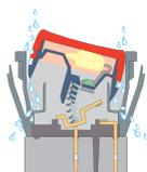
Current carrying parts are protected from moisture. Droplets which may enter the switch are channelled out through ports in the switch body. For IP65 see options below
