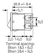
“BC” body w/o barrier primarily for L or R terminals (can be used for all terminals)
