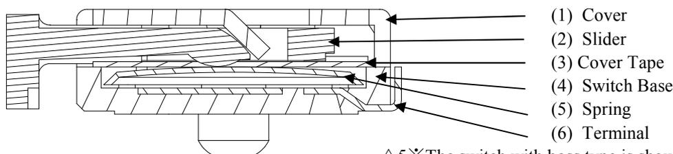
△5※The switch with boss type is shown above as a typical drawing.
