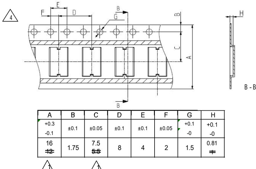
Fig. 12 Carrier tape dimensions
