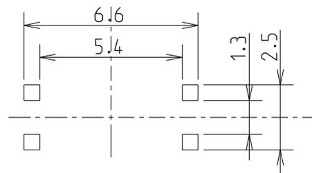
The thickness of solder stencil : 100 μm
