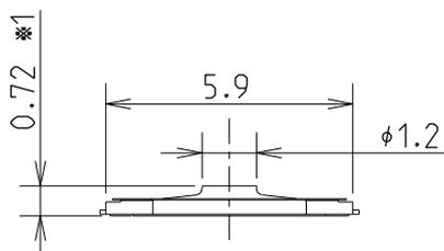
(\*1)The switch height shall be measured with applying 15 gf load.
