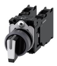
Selector switch, illuminable, 22 mm, round, plastic with metal front ring, white, selector switch, short, 3 switch positions I-O-II, latching, actuating angle 2x45°, 10:30h/12h/13:30h, with holder, 1 NO+1 NC, 1 NO+1 NC, spring-type terminal, with laser labeling, upper case
