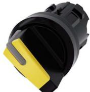
Selector switch, illuminable, 22 mm, round, plastic, yellow, selector switch, short, 2 switch positions O<I, momentary contact type, Actuating angle 45°, 10:30h/12h, with laser labeling, inscription or symbol Customer-specific selection with SIRIUS ACT configurator (CIN)
