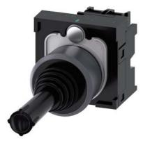
Coordinate switch, 22 mm, round, plastic with metal front ring, black, 2 switch positions, vertical, momentary contact type, without mechanical interlocking in O position, with holder, 1 NO, 1 NO, screw terminal
