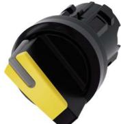
Selector switch, illuminable, 22 mm, round, plastic, yellow, selector switch, short, 2 switch positions O<I, momentary contact type, Actuating angle 45°, 10:30h/12h, with laser labeling, lower case
