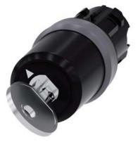
key-operated switch Siemens, 22 mm, round, plastic with metal front ring, lock number SSG10, with 2 keys, 2 switch positions O-I, latching, actuating angle  $90^\circ,\,10:30h/13:30h,$  key removal O, with laser labeling, upper case
