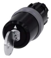
key-operated switch Siemens, 22 mm, round, plastic with metal front ring, lock number SSG10, with 2 keys, 3 switch positions I-O-II, latching, actuating angle 2x45°, 10:30h/12h/13:30h, key removal O, with laser labeling, inscription or symbol customer-specific selection with SIRIUS ACT configurator (CIN)
