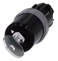
key-operated switch Siemens, 22 mm, round, plastic with metal front ring, lock no. LSG1, with 2 keys, 2 switch positions O<I, momentary contact type, actuating angle 45°, 10:30h/12h, key removal O, with laser labeling, upper case and lower case, always upper case at the beginning of the word
