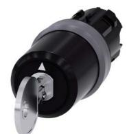
key-operated switch Siemens, 22 mm, round, plastic with metal front ring, lock number SSG10, with 2 keys, 3 switch positions I-O-II, latching, actuating angle 2x45°, 10:30h/12h/13:30h, key removal O+I, with laser labeling, upper case and lower case, always upper case at beginning of line
