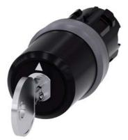
key-operated switch Siemens, 22 mm, round, plastic with metal front ring, lock number SSG10, with 2 keys, 3 switch positions I-O-II, latching, actuating angle 2x45°, 10:30h/12h/13:30h, key removal O, with laser labeling, upper case
