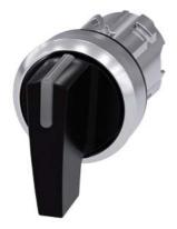
Illuminable selector switch, 22 mm, round, metal shiny, black, Selector switch long, 3 switch positions I>O<II, momentary contact type, actuating angle 2x45°, 10:30 /12 /13:30, Z=50-unit packaging
