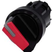
Selector switch, illuminable, 22 mm, round, plastic, red, selector switch, short, 2 switch positions O<I, momentary contact type, Actuating angle 45°, 10:30h/12h, with laser labeling, upper case and lower case, always upper case at the beginning of the word
