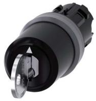
Key-operated switch IKON, 22 mm, round, plastic with metal front ring, lock number 360012K1, with 2 keys, 3 switch positions I-O-II, latching, actuating angle 2x45°, 10:30h/12h/13:30h, key removal O, with laser labeling, lower case
