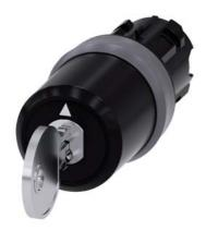
Key-operated switch BKS, 22 mm, round, plastic with metal front ring, lock number S1, with 2 keys, 3 switch positions I-O<II, left latching, right momentary contact type, actuating angle 2x45°, 10:30h/12h/13:30h, key removal I, with laser labeling, lower case
