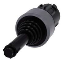
Coordinate switch, 22 mm, round, plastic with metal front ring, black, 2 switch positions, vertical, momentary contact type, with mechanical interlocking, with laser labeling, upper case and lower case, always upper case at the beginning of the word
