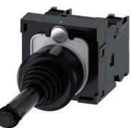
Coordinate switch, 22 mm, round, plastic, black, 2 switch positions, horizontal, momentary contact type, with mechanical interlocking in O position, with holder, 1 NO, 1 NO, screw terminal
