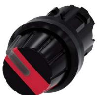
Selector switch, illuminable, 22 mm, round, plastic, red, Rotary knob, 2 switch positions O-I, latching, actuating angle 90°, 10:30h/13:30h, with laser labeling, upper case
