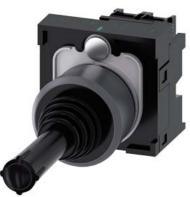
Coordinate switch, 22 mm, round, plastic with metal front ring, black, 2 switch positions, vertical latching, without mechanical interlocking, in O position, with holder, 1 NO, 1 NO, screw terminal, Z=20-unit packaging
