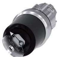
Key-operated switch IKON, 22 mm, round, metal, shiny, lock number 360012K1, with 2 keys, 2 switch positions O-I, latching, actuating angle 90°, 10:30h/13:30h, key removal O, with laser labeling, inscription or symbol Customer-specific selection with SIRIUS ACT configurator (CIN)
