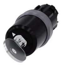
Key-operated switch BKS, 22 mm, round, plastic with metal front ring, lock number S1, with 2 keys, 2 switch positions O<I, momentary contact type, Actuating angle  $45^{\circ}$ , 10:30h/12h, key removal O, with laser labeling, upper case
