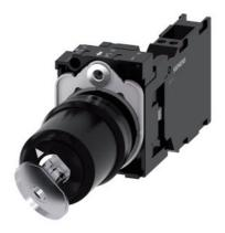
key-operated switch Siemens, 22 mm, round, plastic, lock number SSG10, with 2 keys, 2 switch positions O-I, latching, 10:30h/13:30h, key removal O+I, with holder, 1 NO+1 NC, spring-loaded terminal, with laser labeling, upper case and lower case, always upper case at beginning of line
