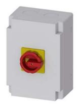
SENTRON, Switch disconnector 3LD, emergency switching-off switch, 6- pole, lu: 63 A, operating power / at AC-23 A 400 V: 22 kW, Molded plastic encapsulation for metric cable gland, 1 NC, 1 NO, rotary operating mechanism, red/yellow
