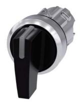
Illuminable selector switch, 22 mm, round, metal shiny, black, Selector switch long, 3 switch positions I-O-II, latching, actuating angle 2x45°, 10:30 /12 /13:30, Z=50-unit packaging
