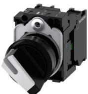
Selector switch, illuminable, 22 mm, round, plastic, white, selector switch, short, 2 switch positions O-I, latching, 10:30h/13:30h, with holder, 1 NO, 1 NC, screw terminal, with laser labeling, inscription or symbol Customer-specific selection with SIRIUS ACT configurator (CIN)
