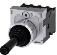
Coordinate switch, 22 mm, round, metal shiny, black, 4 switch positions, momentary contact type, with mechanical interlocking, in O position, with holder, 1 NO, 1 NO, 1 NO, 1 NO, screw terminal,
