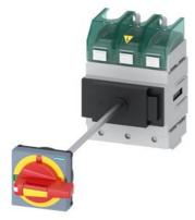
SENTRON, Molded case switch 3LD5 UL, Emergency switching-off, 3-pole, certified according to UL489 UL60947-4-1 and IEC60947-3, UL: 125A, SCCR 65kA at 480VAC, Operating power at 480VAC 3-phase: 75hp, IEC: 125A, Operating power at AC-23A at 400V: 55kW, floor mounting with door coupling rotary operating mechanism, defeatable, emergency switching-off, 4-hole mounting of the handle, without tolerance compensation, incl. terminal covers for the infeed side
