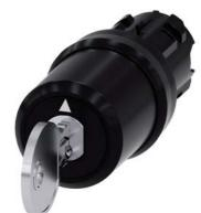
Key-operated switch BKS, 22 mm, round, plastic, lock number S1, with 2 keys, 3 switch positions I-O<II, left latching, right momentary contact type, actuating angle 2x45°, 10:30h/12h/13:30h, key removal O+I, with laser labeling, upper case and lower case, always upper case at beginning of line
