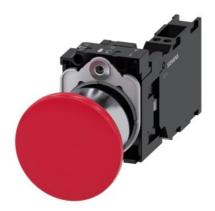
Mushroom pushbutton, 22 mm, round, metal, shiny, red, 40mm, latching, pull-tounlatch mechanism, with holder, 1 NO+1 NC, spring-type terminal, with laser labeling, inscription or symbol Customer-specific selection with SIRIUS ACT configurator (CIN)
