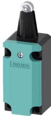
Position switch Metal enclosure 40 mm according to EN 50041, Device connection 1x (M20 x 1.5) 1 NO/1 NC quick action contacts, roller plunger with 3 mm overtravel and stainless steel roller 13 mm
